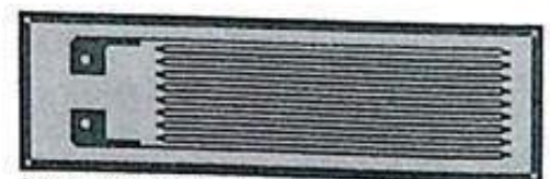
Wire strain gauge bonded on elastic backing Fig. 6.3
